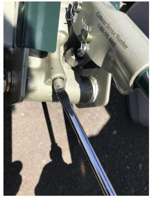
o Test functionality by pumping the rod up and down to see if the jack raises.
