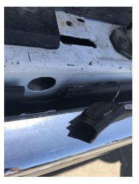
o Insert lowering rod into hole to the lower mechanism to rotate counterclockwise.
